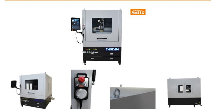
The C1 is a self contained CNC router. The 'one-box' design has a compact footprint which incorporates conventianly located CNC controler, storage is also intergrated into the design with 4 convenient drawers to store all of the machine's tools and accessories... and there is even space to store the vacuum pump under the table.
