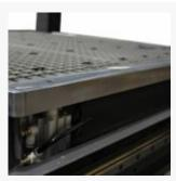
**Pop up location pins** Pnuematic pins to assist you with your workpiece alignment.
