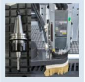
**Quick release tool holder** -For a quick swap to a new tool, press the button and the tool pop out.
