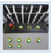
**Pneumatic Solenoid actuated vacuum zones** -Control isolated vacuum zone locations with the press of a button.
