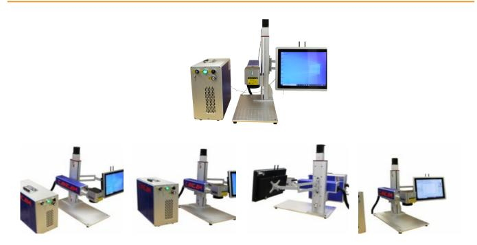
The OP-FML is a (open frame fiber marking laser system) that is designed to be stationary and offers high precision even in high volume operations at powers as high as 100 watts with minimal down time. This design allows for larger pieces to be places underneath the galvo scanner with the press of a button due to the built in Z axis motor.
