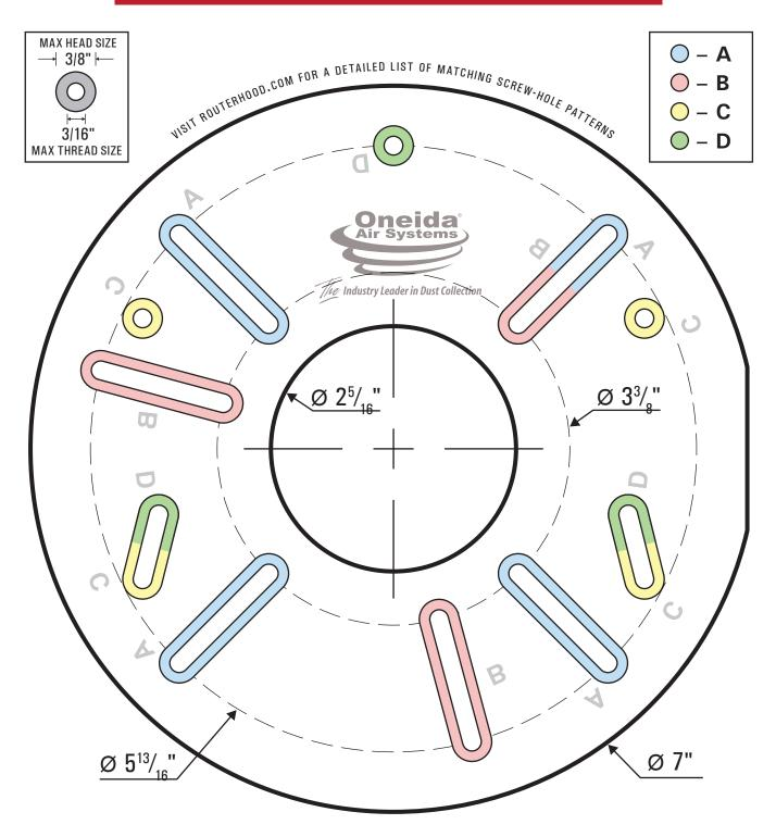
In addition to confirming screw hole compatibility, ensure that your router base has a center hole diameter of at least 2 3/8". A router base with a smaller center hole will not work with the Dust-Free Router Hood.
