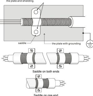
Remove any paint on metal saddle for good ground contact with the plate and shielding.
