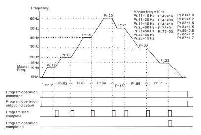
Note: The above diagram shows one complete PLC cycle. To restart the cycle, turn the PLC
