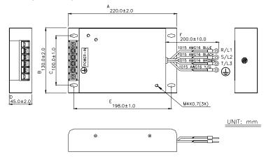
EMI Filter (40TDS4W4B) Used on 5-7.5 HP/230V Three Phase Models.
