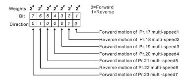
The setting value=bit7 x  $2^6$ +bit6 x  $2^5$ +bit5 x  $2^4$ +bit4 x  $2^3$ +bit3 x  $2^2$ +bit2 x  $2^1$ +bit1 x  $2^0$ = 0 x  $2^6$ +1 x  $2^5$ +0 x  $2^4$ +0 x  $2^3$ +0 x  $2^2$ +1 x  $2^1$ +0 x  $2^0$ = 0+32+0+0+0+2+0+0 = 34
