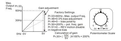
In this example, a 6 Hz (10% of 60 Hz) negative bias is used. This setting is used to provide a noise margin (1V in this example) in noisy environments. Note that the top frequency is reduced to 54 Hz.
