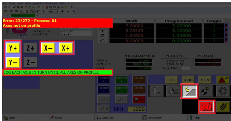
Fig. 5.5 Returning axes to profile.
