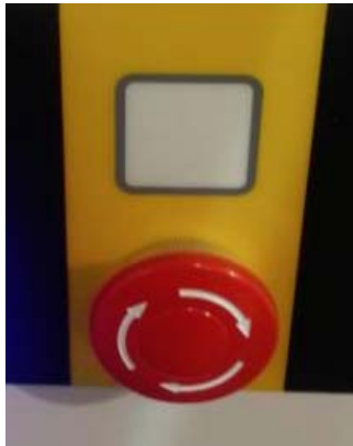
Fig. 2.7 Turn E-STOP and click “E-Stop Reset” to clear E-Stop fault.
