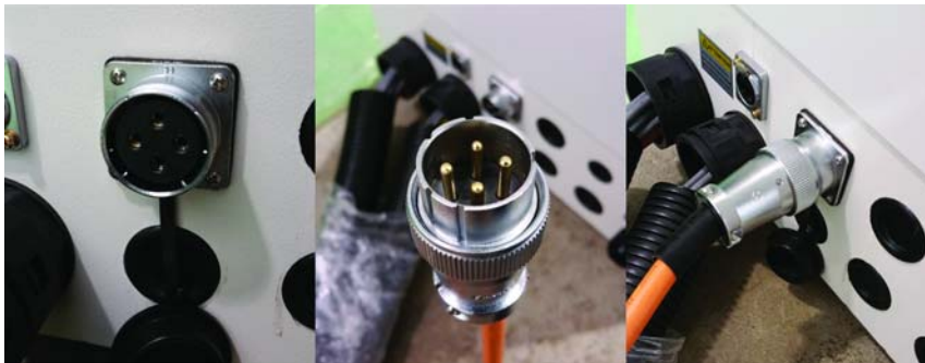
Fig. 1.8 Connecting vacuum pump to electric cabinet.
