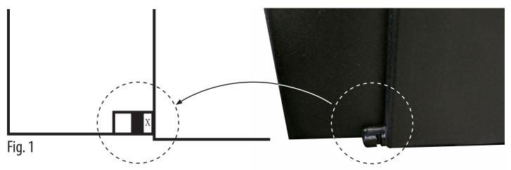
Using a sharp wood chisel, a hand grinder, or other suitable tool, carefully trim off the inside of the lug where indicated by the "X" in Fig. 1. First remove a small amount of material and then test the fit. Repeat as necessary until the clamp locks securely. Repeat the procedure on the opposite lug until the clamp on that side locks securely. Fig. 2 shows a completely trimmed lug.
