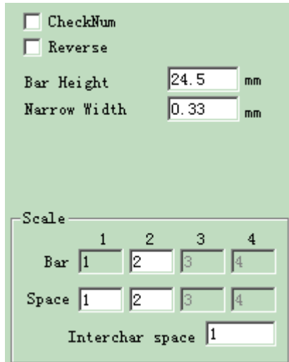
Figure 4-16 One-Dimensional Barcode Parameter Setting
